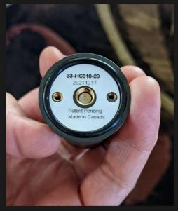
This is the view of the bottom of the antenna. Note the male connector.
