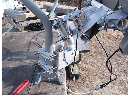
Figure 2. Azimuth/elevation mount using 2 DiSEqC SG2100 motors
