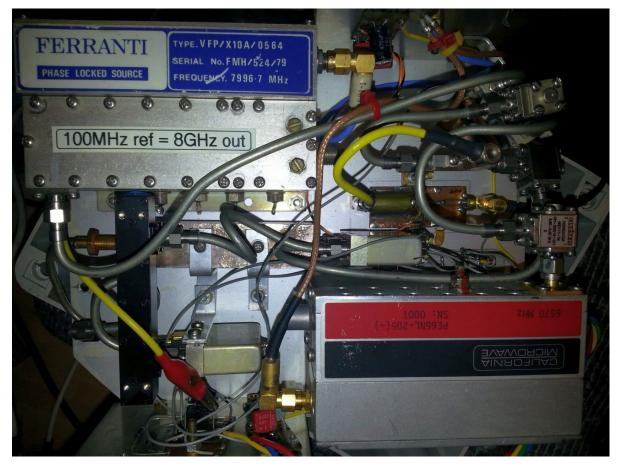
This is the current dual-band X-Band converter in use at UHF-Satcom; a pair of DF9NP PLL oscillators running at 3.5GHz and 4GHz, both of which are doubled using a FET doubler followed by a tight filter to give 7GHz and 8GHz LO's which are switched into the mixer. Front end filters are switched giving access to mil-sat or DSN bands:
