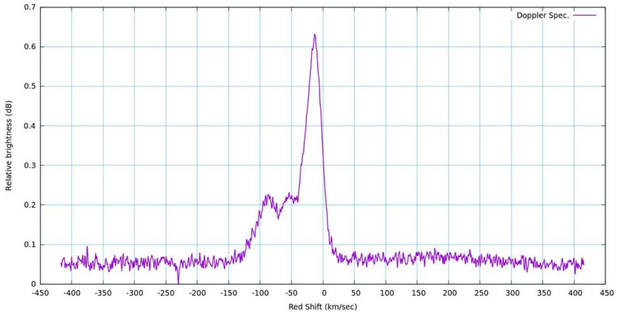
The resulting SNR was much improved and the signal peak was almost 0.4dB higher, which put it much closer to what one would expect given the aperture.
