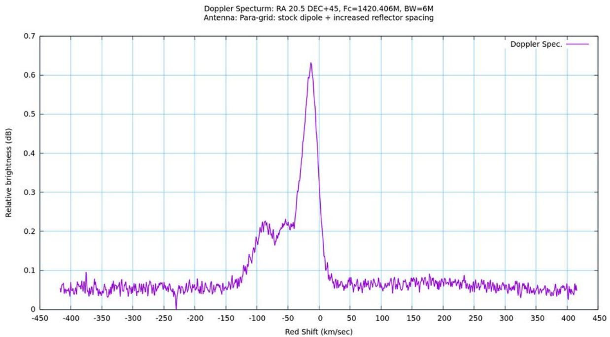
The resulting SNR was much improved and the signal peak was almost 0.4dB higher, which put it much closer to what one would expect given the aperture.
