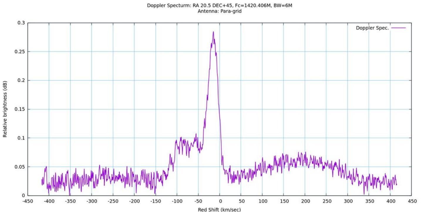
This was certainly adequate for an initial observation, but theoretically (given the effective aperture of this 30cm x 60cm parabola) the response should have been better.
