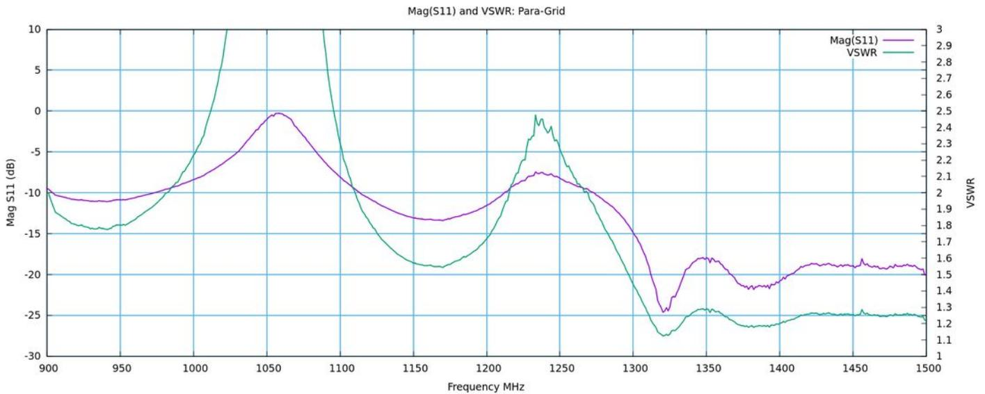
The VSWR shown by the “as manufactured” feed dipole at 21cm wavelength is actually quite acceptable at 1.3:1. This suggested that another “sky test” should be performed with the feed restored to “as manufactured” condition.
