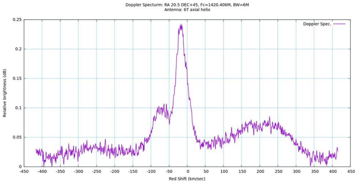
The SNR is poor, and the peak sky response is a paltry 0.25dB above the noise.
