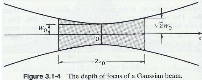
Figure 3.1-4 The depth of focus of a Gaussian beam.
