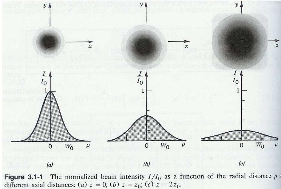
**Figure 3.1-1** The normalized beam intensity  $I/I_0$  as a function of the radial distance  $\rho$  at different axial distances: (a)  $z = 0$ ; (b)  $z = z_0$ ; (c)  $z = 2z_0$ .
