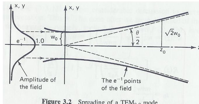
Figure 3.2 Spreading of a TEM<sub>0,0</sub> mode.
