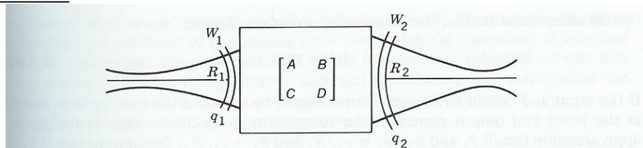
**Figure 3.2-9** Modification of a Gaussian beam by an arbitrary paraxial system described by an ABCD matrix.
