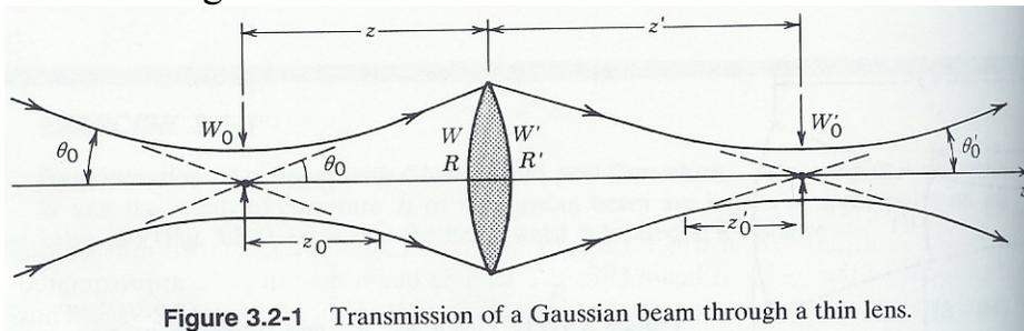
**Figure 3.2-1** Transmission of a Gaussian beam through a thin lens.
