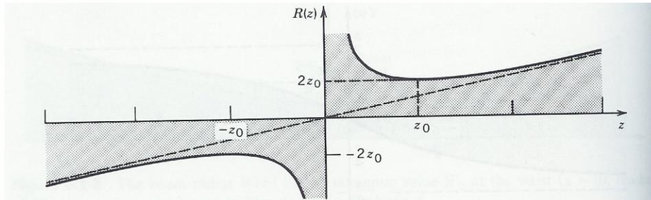
**Figure 3.1-6** The radius of curvature  $R(z)$  of the wavefronts of a Gaussian beam. The dashed line is the radius of curvature of a spherical wave.
