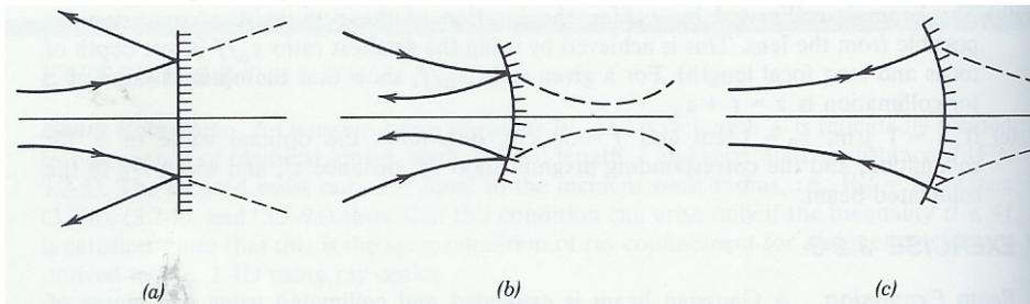
**Figure 3.2-8** Reflection of a Gaussian beam of curvature  $R_1$  from a mirror of curvature  $R$ : (a)  $R = \infty$ ; (b)  $R_1 = \infty$ ; (c)  $R_1 = -R$ . The dashed curves show the effects of replacing the mirror by a lens of focal length  $f = -R/2$ .
