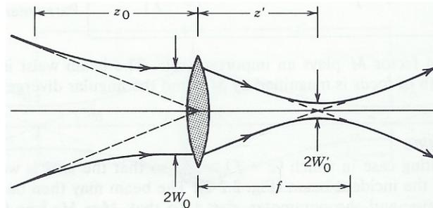
**Figure 3.2-3** Focusing a beam with a lens at the beam waist.
