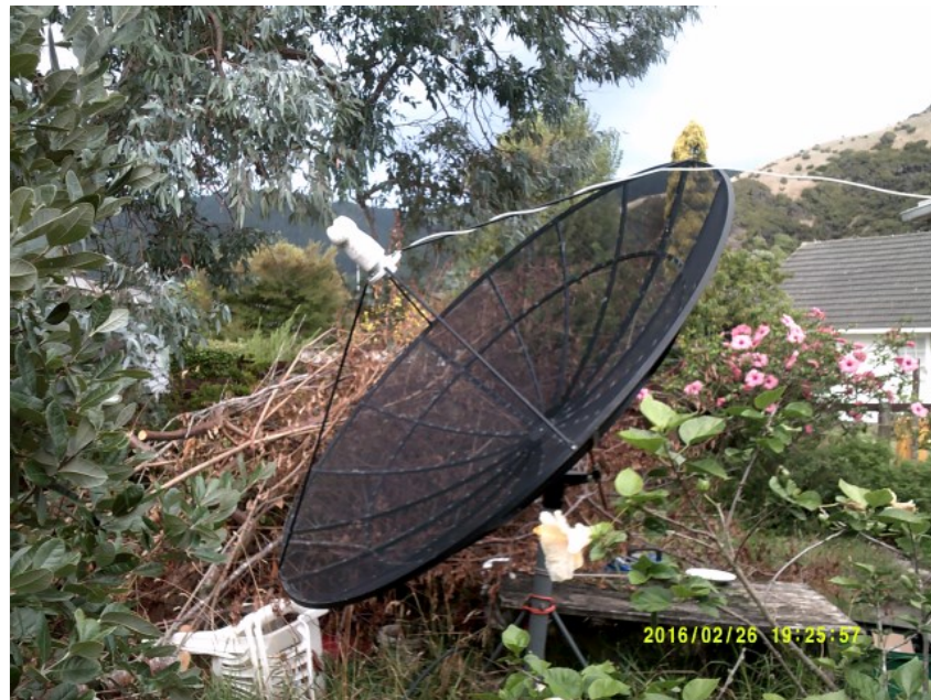
New PLL LNB on 2.3m dish
