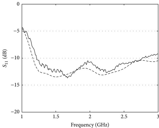
FIGURE 7: Reflection coefficient ( $S_{11}$ ) against frequency of the proposed strip-helical antenna. Solid line: measured data; dashed line: simulated data.
