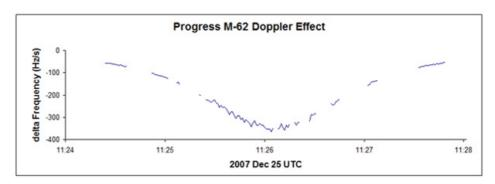
This plot shows the rate of change in frequency as time passed. The missing segments are the result of variations in signal strength.
