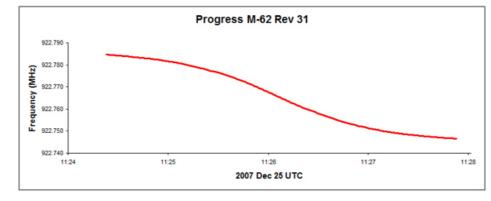
Here is the Doppler curve for Progress M-62 on rev 31, 2007 December 25 as viewed from Lincoln in the UK. It exhibits a classic low-orbit "S" shape and the time of closest approach to the receiving station comes in the middle of the nearstraight section, just after 11:26 UTC. Data was collected as an output stream from an SDR-14 Software Derived
