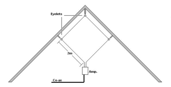
No rocket science here; I simply screwed three eyelets in the rafters to give an approximate diamond shape. Since my house is facing due N/S, the eyelets were placed that the direction of the loop is pointing NE/SW.
