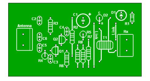
Probably a neater way of doing it would be to paste a parts-placement overlay to the board first. It's just a matter of then stuffing all the components where they are shown.
