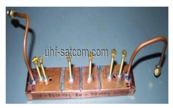
The waveguide filter described above has made about a 4 to 5 dB improvement in the received signal, presumably due to the removal of the image noise. The two images below show the down converter with added filter, and the improvement in received signal. The probe is further away today, at 4.17 million miles.
