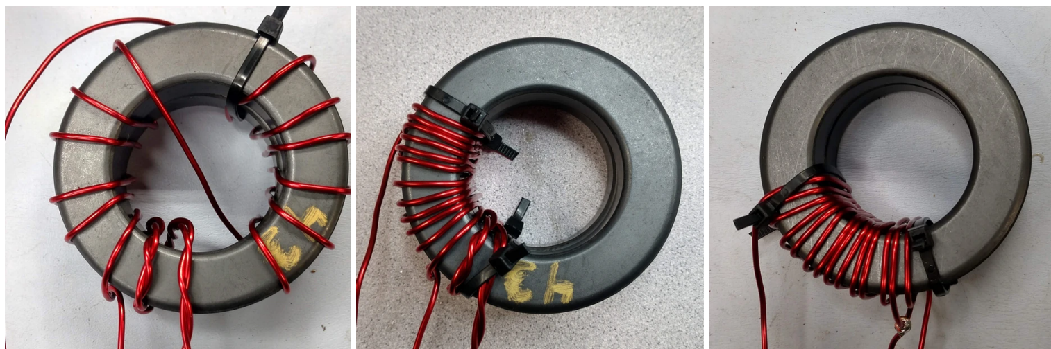
Figure 1 L to R Twisted Primary w/ Crossover, Twisted Primary w/ No Crossover, Tapped Single Winding
