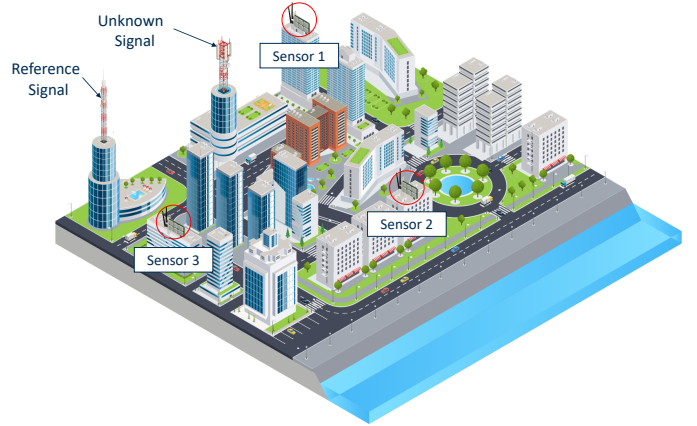
Fig. 1. Unknown transmitter can be localized collaboratively by using a network of sensors that make use of a reference signal transmitter to synchronize among them
